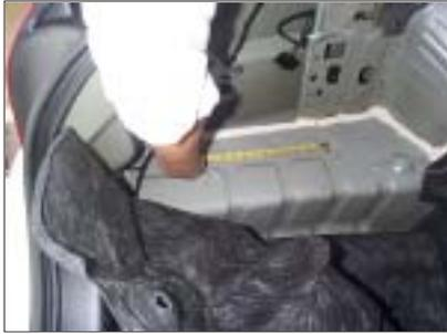
Measure 6-5/16" back from the center of the first hole, get the center point of the second hole and use 17/64 metal drill bit to make a hole.
