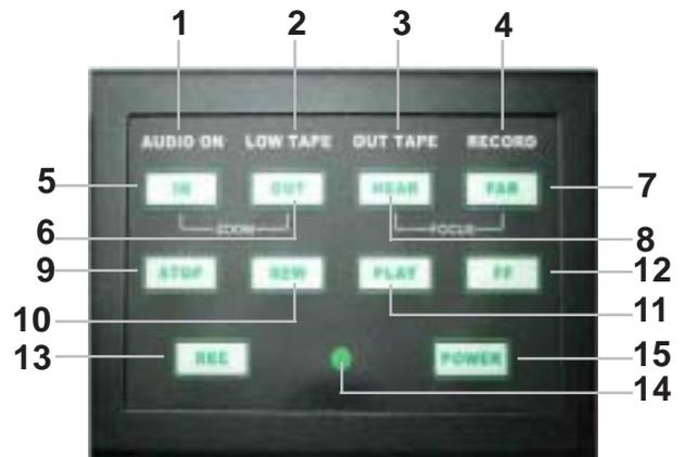
Figure 10 : Bottom of Control Head
