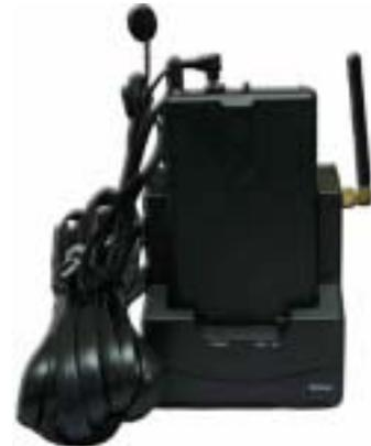
Figure 8 : 900MHz Spread Spectrum Transmitter & Reciever / Charging Base
