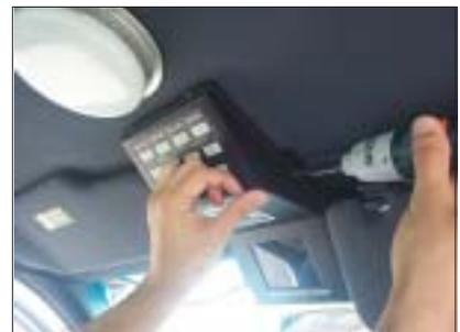
View of control head being mounted with wires already attached to connections
