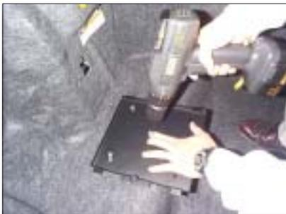
Place a hex head sheet metal screw at the middle hole of mounting plate.
